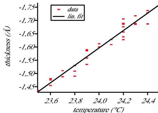
FIG. 3. (Color online) Linear drift of the surface plasmon plotted as thickness change ( $n=1.5$  in water  $n=1.33$ ) dependent on the temperature ( $^{\circ}$ C) over a time period of 5.5 h. Linear least-squares line fit results in an average thickness error of 0.33 Å per  $^{\circ}$ C. Red dots: measured data, black line: linear fit.
