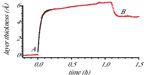
FIG. 2. (Color online) Binding kinetics of cysteamine layer on gold. (A) Start of the absorption. (B) Rinse with PBS. The thickness of  $d=4.8$  Å is measured between points (A) and (B). The index of refraction of the cysteamine layer was assumed to be  $n=1.525$ . The black line is a guide for the eye.
